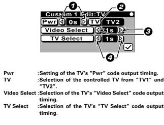
Check the operation after setting the time. If macro play does not occur, increase the time settings with the following procedure.
